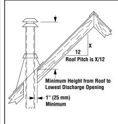
Figure 4 - Vertical Vent Termination Clearances
